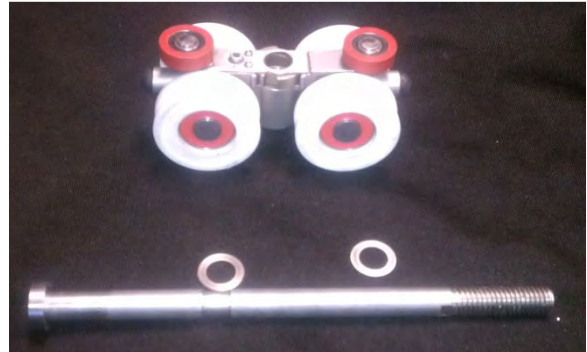
BFH-04 intermediate roller assembly
