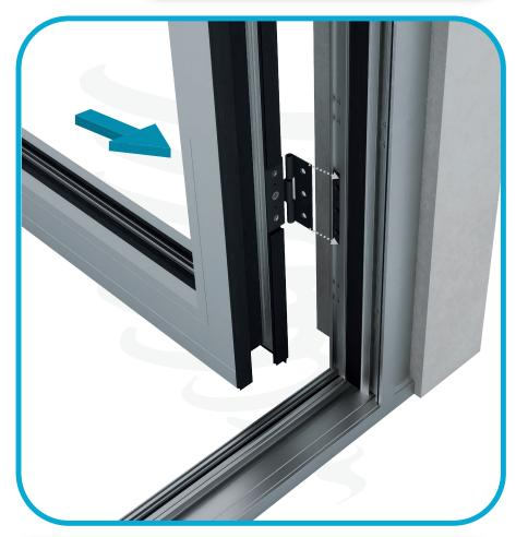
Carefully place the door back into the frame, aligning the hinges with their corresponding positions. Use two people to lift and position the door to prevent damage or injury. Make sure the door is properly seated before proceeding.
