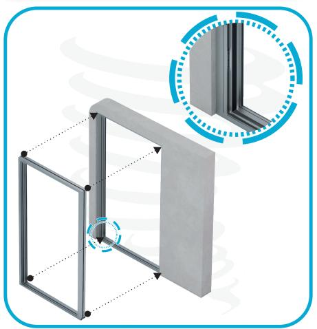
Carefully remove both adjustable jambs from the frame, including the one located on the door strike side. Handle with care to avoid bending or damaging the aluminum profiles.
