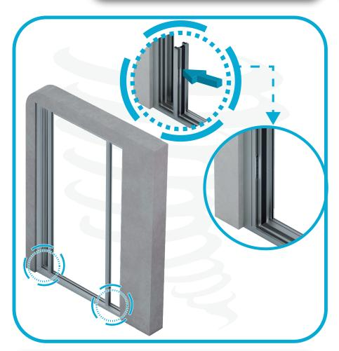
Reposition both adjustable jambs back into the frame, ensuring they are fully seated and properly aligned.
