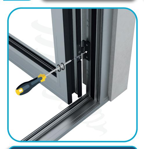
After the door is properly aligned and level, install the DIN 7981 Z screws in all hinges
