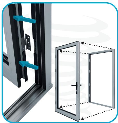
Carefully lift and remove the door from the frame once all hinge screws have been removed. Make sure to support the weight of the door to prevent
