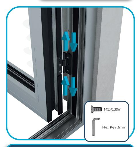
Once the door is installed and secured, slightly loosen the M5 x 0.39" hinge screws to allow vertical adjustment as needed. The door can be adjusted up to 1/4" to achieve proper alignment.
