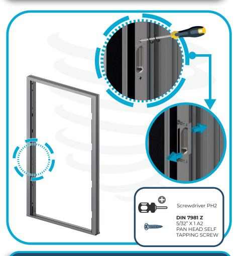
To adjust the lock latch, slightly loosen the DIN 7981 Z screws that secure the latch plate. This will allow the latch to be moved horizontally to achieve the correct alignment with the strike. Once the desired position is reached, retighten the screws firmly to secure the latch in place.
