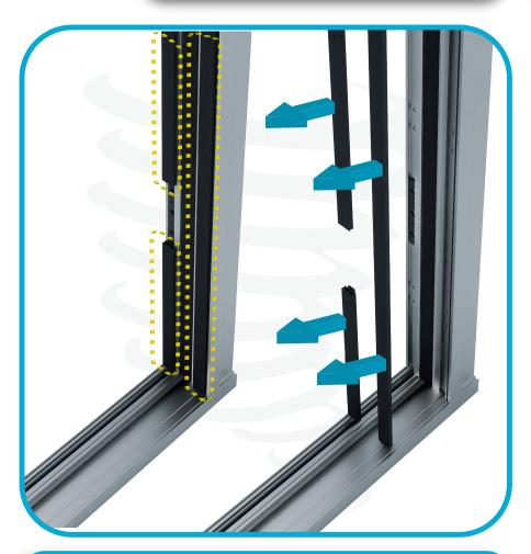
With the frame clear, remove the weather seals attached to the adjustable jamb.
