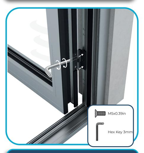
Install the M5  $\times$  0.39" screws into the frame-side hinges to firmly secure the door.
