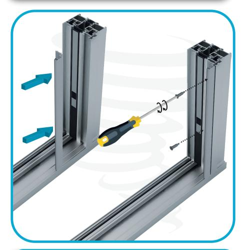
Place the T-astragal on the interior side of the door. Secure it in position using DIN 7981 Z screws. Ensure all screws are properly seated without over-tightening to maintain proper alignment.
