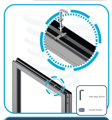
Use a 3 mm hex key, adjust the top adjustment ("butterfly") to fine-tune the vertical alignment of the door once it is re-hung.
