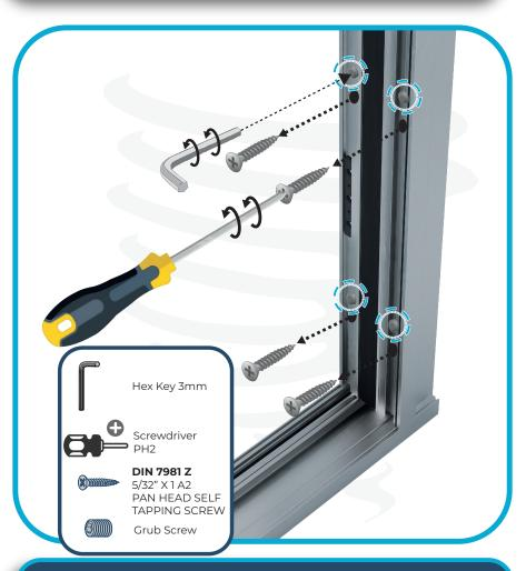
Using a 3 mm hex key, loosen the grub screws, and using a PH2 Phillips screwdriver, remove the DIN 7981 Z screws located on the adjustable jamb.
