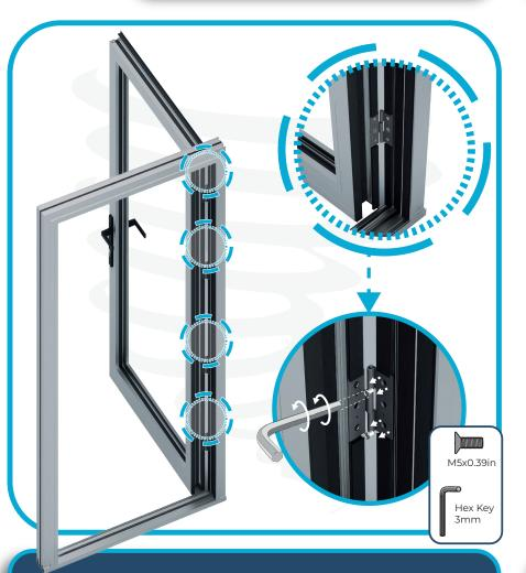
Using a 3 mm hex key, remove the M5 X 0.39" screws located on the jamb-side hinges.
