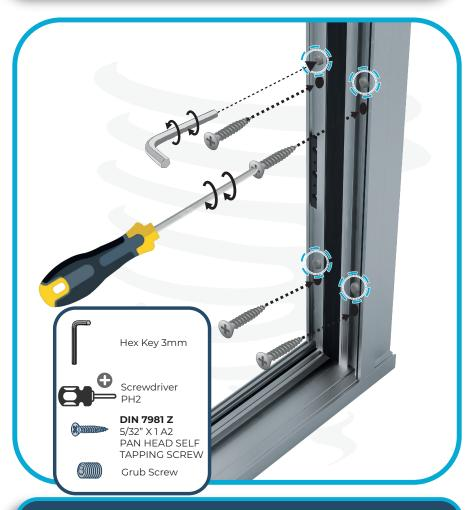
Use a 3 mm hex key to tighten or loosen the grub screws as needed.
