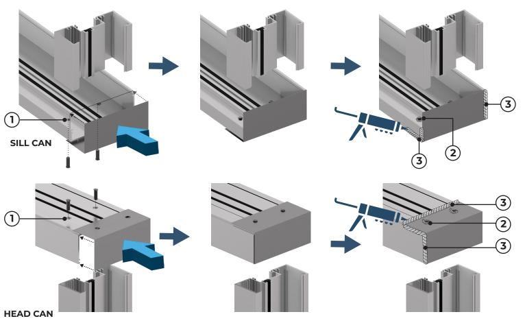
Clean all surfaces prior to applying sealants. See sealant manufacturer requirements.
