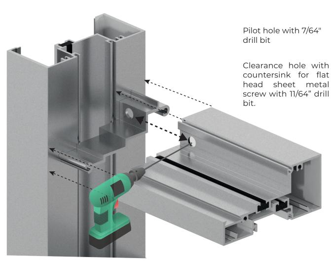
Use a countersink bit for flat head screws (usually 82° angle).
